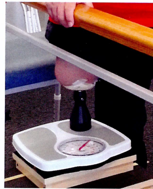
LEFT: Initial use of an abutment attached to the OGAAP-OPL in order to load weight
